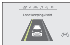
When the front-view camera detects the vehicle moving outside of the lane being traveled in, a yellow indicator will illuminate either on the left or right lane (shown in both images above)
