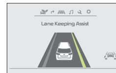
When the front-view camera detects the vehicle moving outside of the lane being traveled in, a yellow indicator will illuminate either on the left or right lane (shown in both images above)
